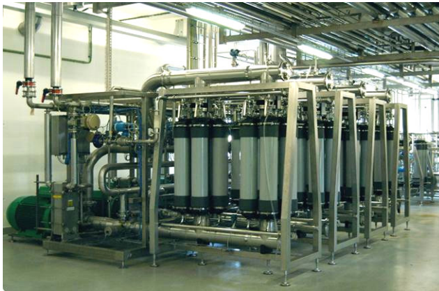
Clarification system for 5000 L/h
