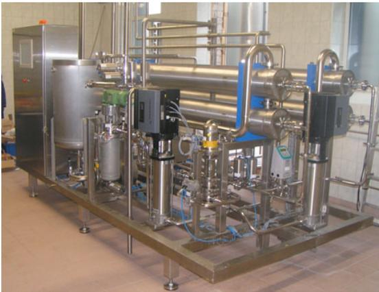
The **MMS Swissflow** RO systems enable the reduction of high BOD waste streams, by producing clean water and a concentrated whey/lactose stream for animal feed. The concentrate whey/lactose reduces whey volumes by 4 fold, resulting in a substantial reduction in transportation costs.
