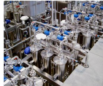
**MMS** produce a range of **SwissFlow** RO systems capable of handling feed rates from 1'000 – 20'000 l/h. The capacity of the system is a function of several parameters, including feed concentration, level of retentate concentration and operating temperature. With our specialists we will enable you to select the correct system for your product and processing requirements.
