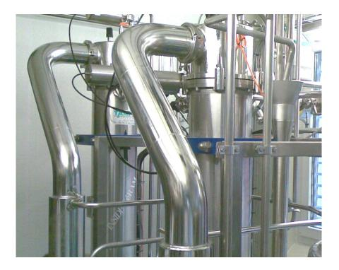
The **MMS** SwissFlow MF systems enables the reduction of bacterial count in permeate by a physical barrier. The operation is conducted at low operating temperatures (50 °C) producing near to native product quality. The systems are designed for minimum dead volumes, and offer high permeate yields. The retentate can be further heat treated to recover all the value in your milk.
